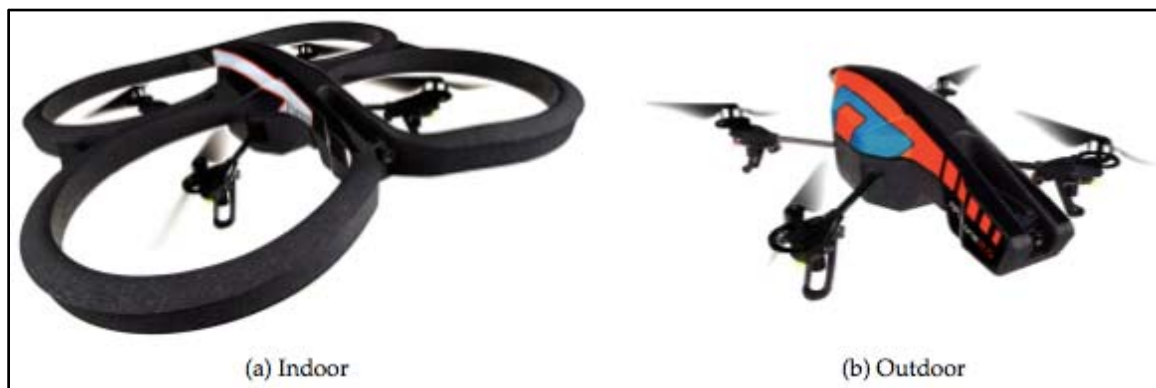
Figure 1. AR Drone 2.0 (from [17])
