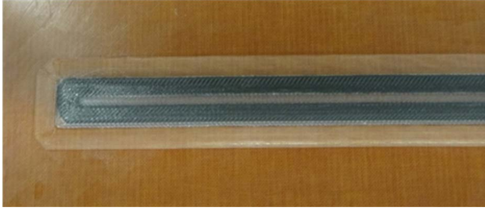
Figure 5. Close-Up View of Continuous Carbon Fiber Composite
