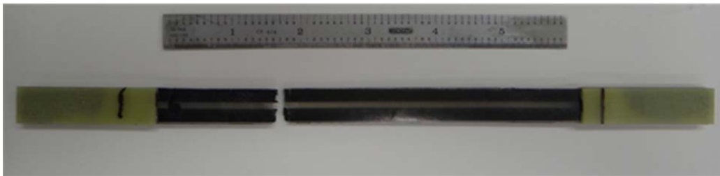
Figure 6. Continuous Carbon Fiber Composite Specimen After Testing
