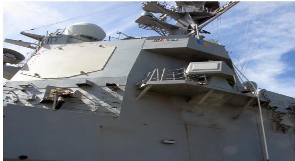
U.S. Navy installed the Lockheed Martin SEWIP Block 2 System on DDG-96 for operational testing over
