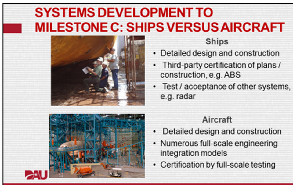
Figure 6. Differences Between Ships and Aircraft at the Systems Development Phase
