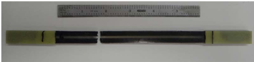
Figure 6. Continuous Carbon Fiber Composite Specimen After Testing
