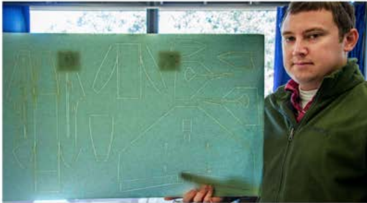
Figure 1: LT Ryan Beall used a laser cutter to rapid prototype a glider to test performance of a guidance control system he designed and built.
