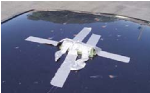
Figure 4. An Example of How the RFID Tags Were Placed (Note: This tag was placed on the roof of the vehicle and secured with Duct Tape.)
