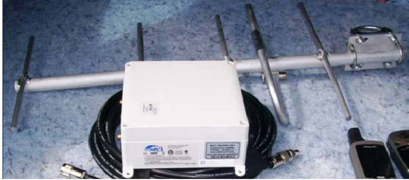
Figure 2. Photograph of One of the Antennas Used in the Test
