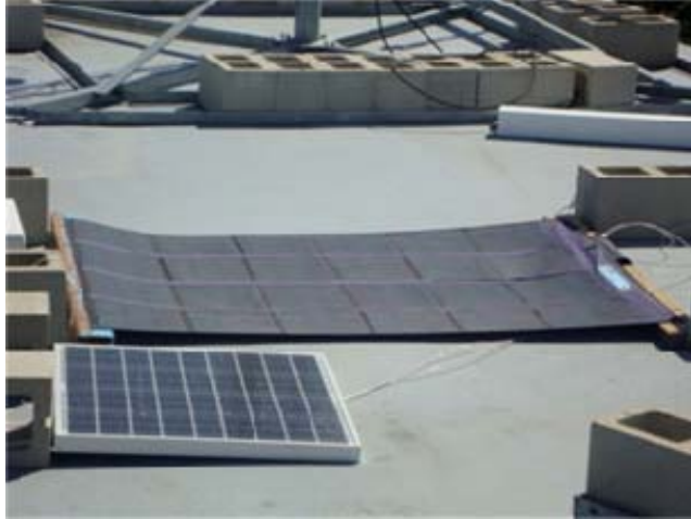
Figure 23. The Two Solar Panels Utilized for the Wind-PV Experiment (Note: The Kyocera panel is in the foreground and the PowerFilm panel is in the background.)
