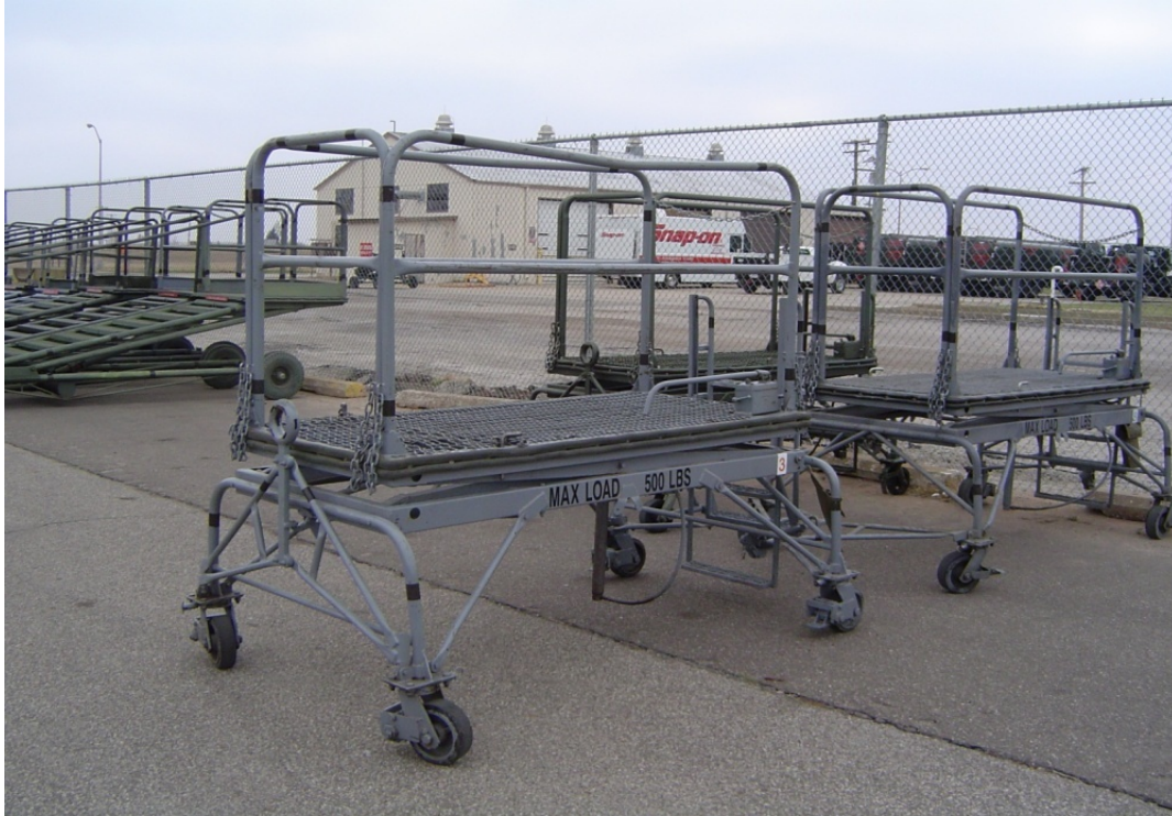
Figure 2. B-4 Maintenance Stand
