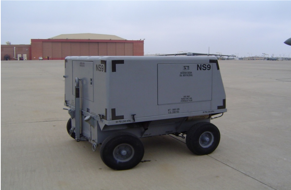
Figure 9. Nitrogen Service Cart
