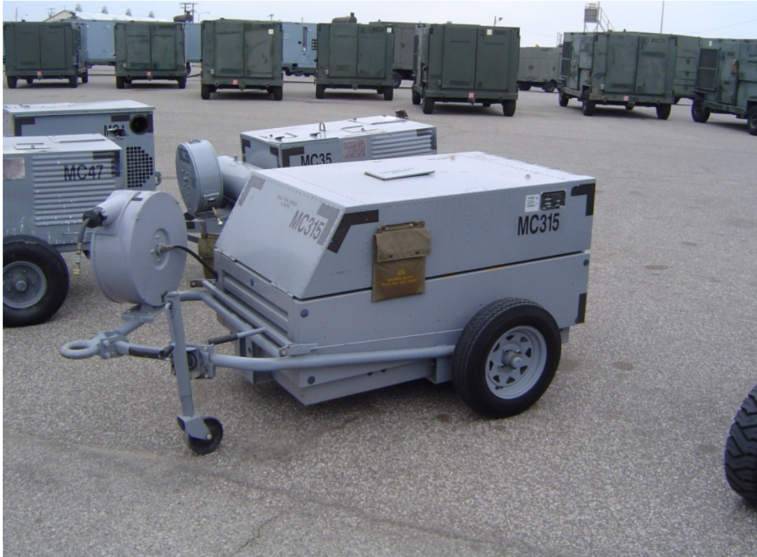
Figure 8. Low Air Compressor
