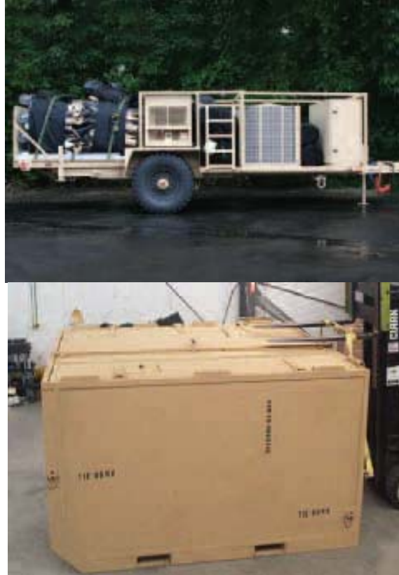
Figure 37. DRASH Trailer Mounted Support System and Optional Shipping Container
