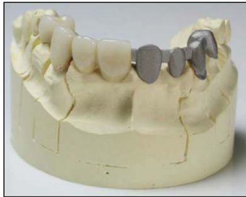
Figure 5. Dental Implants Made From CAD File Using DMLS (Overton, 2009, p. 45)
