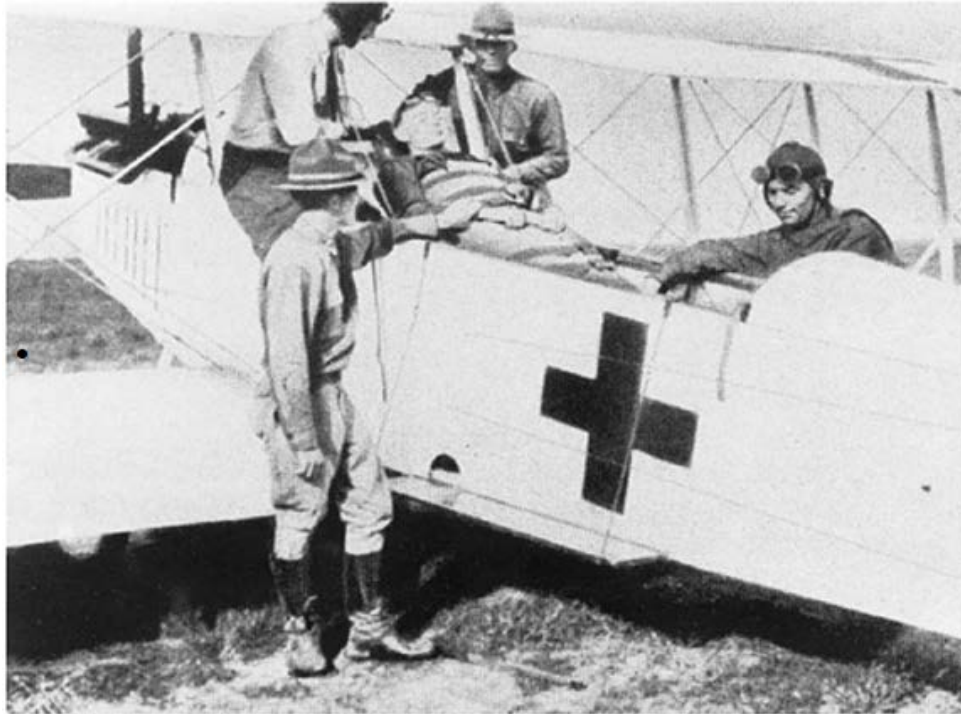
Note. The Curtiss JN-4 Jenny was transformed into an air ambulance by removing the rear seat Figure 7. The Curtiss JN-4 Jenny (from Hurd et al., 2002, p. 7)
