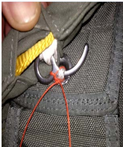
Figure 13. Main Curve Pin Safety Tie. Source: Army Airborne Board (2016).
