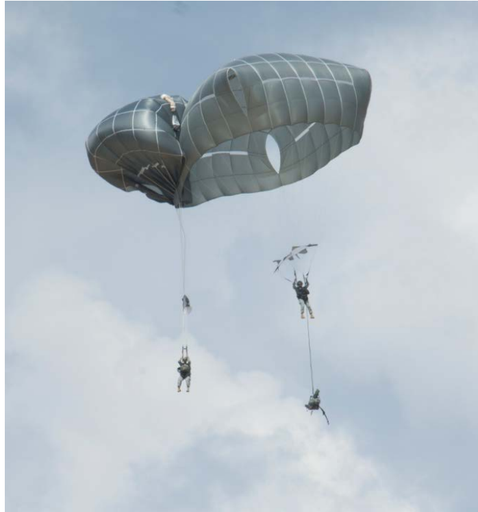
Figure 11. T-11 Corner Vent Entanglement. Source: Duncan (2016).
