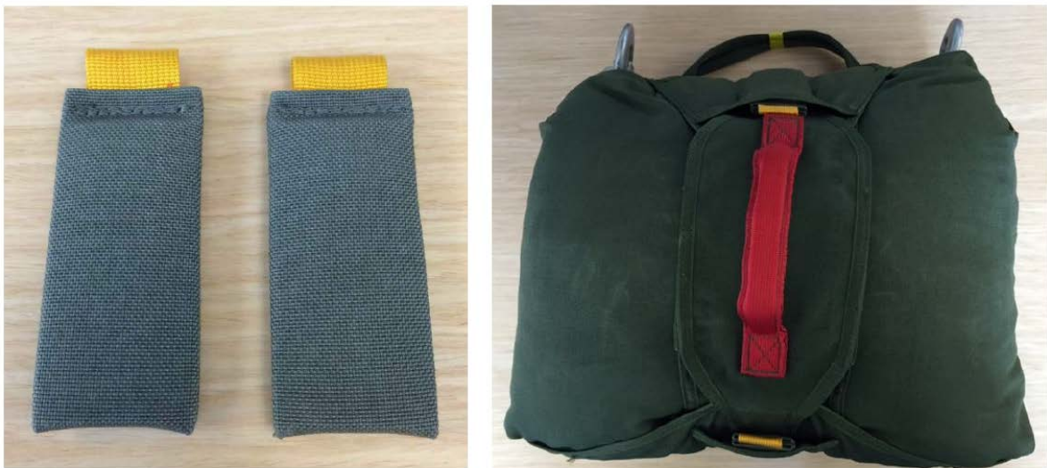
(L) Shows the inserts and the (R) shows inserts on the original T-11R pack tray.
