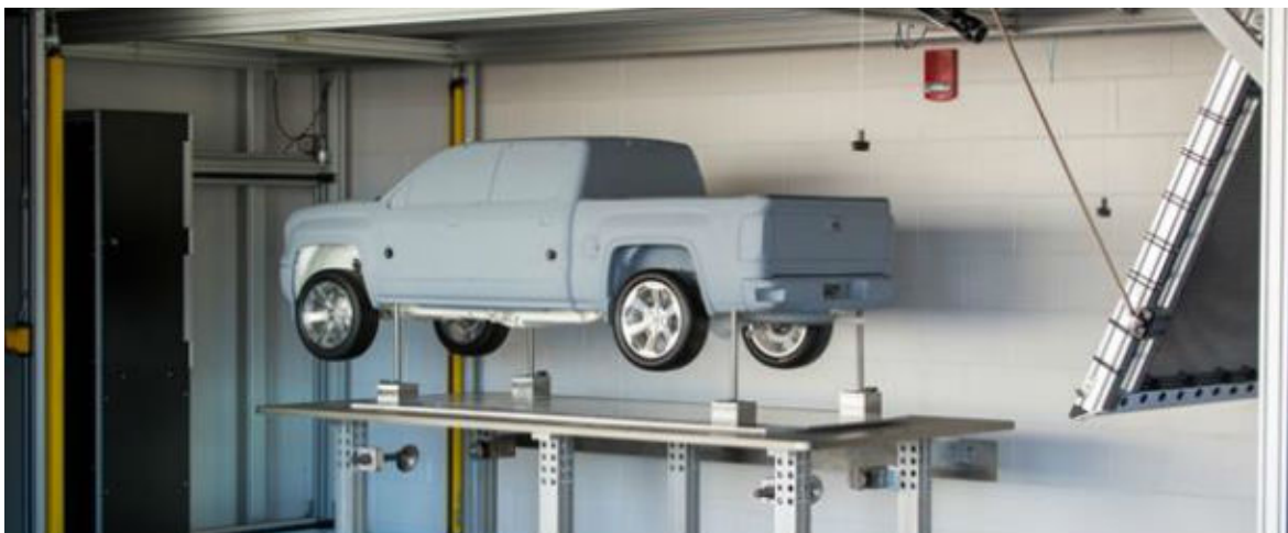
Figure 5. A 3D-Printed 40%-Size Model of a GM Truck Created for Wind Tunnel Testing. Source: Helsel (2015).
