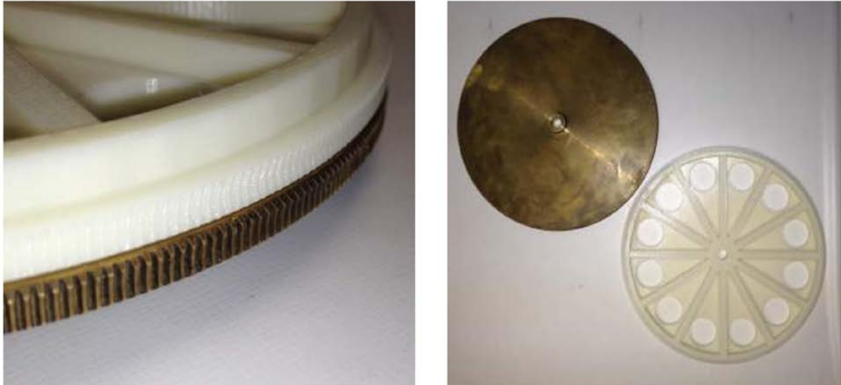
Figure 7. 3D-Printed Replica Next to the Original Part TE-779 Test Fixture Used for Testing H-53 Stick Position Sensors Source: Lukesh, personal communication (2016).
