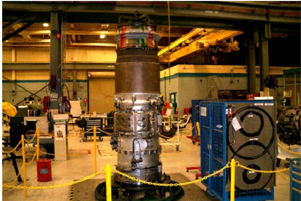
Figure 20. Joint Cold and Hot Sections at the External Build-Up Pit. 84
