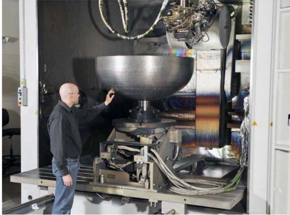
Figure 4. The EBAM Metal 3D Printer at Lockheed Martin's Manufacturing Facility Located in Littleton, CO. Source: Grunewald (2016).
