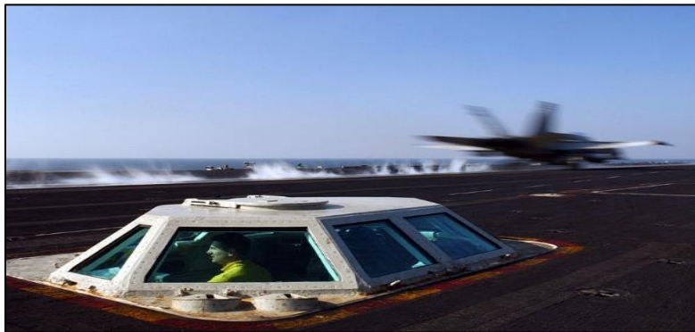
Figure 2. Aircraft shooters watch from inside the ICCS. Source: Official website of the United State Navy page (2018).
