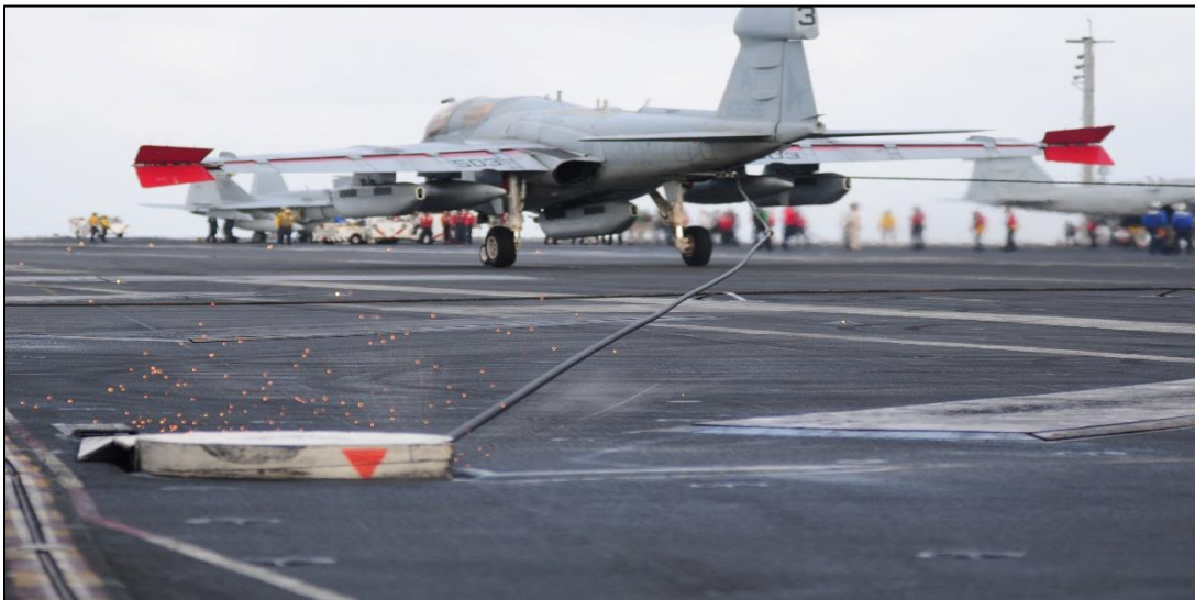
Figure 4. An EA-6B Prowler, assigned to the "Rooks" of Electronic Warfare Squadron One Three Seven (VAQ-137), catches one of four arresting wires on the flight deck of the aircraft carrier USS Enterprise (CVN 65). Source: NAVAIR (2018).
