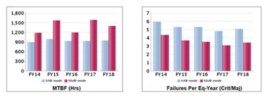
Figure 6. NSWC CIWS Reliability Metrics. Adapted from Naval Surface Warfare Center (2018).
