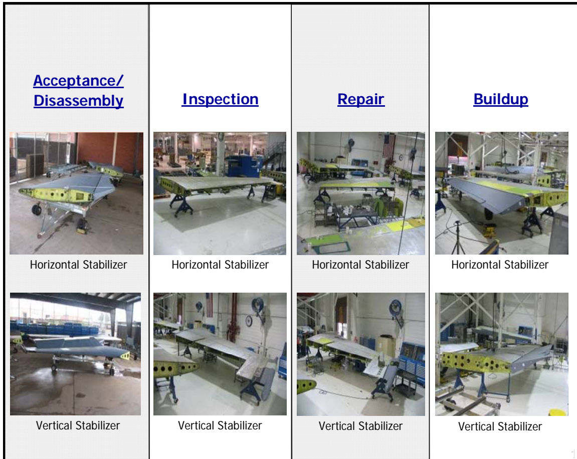
Figure 3. HV Repair Cell Model's Four Milestones
