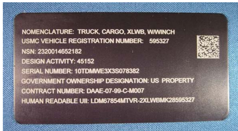
Figure 4. Example of an Anodized Aluminum Data Plate
