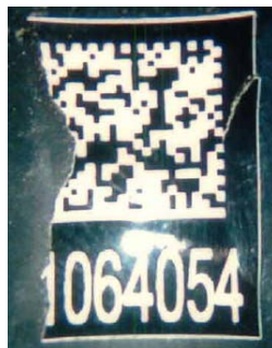
Figure 25. TESA Tape after Environmental Testing
