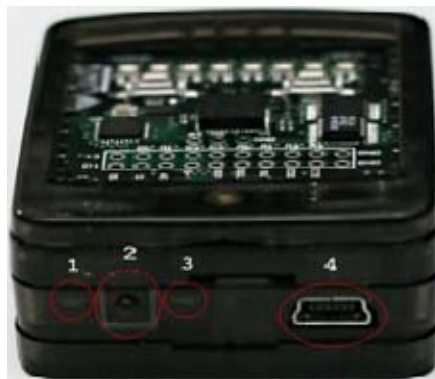
Figure 12. SunSPOT USB Connection used to Load SDK and Recharge Internal Battery (SunSPOT World, 2009)
