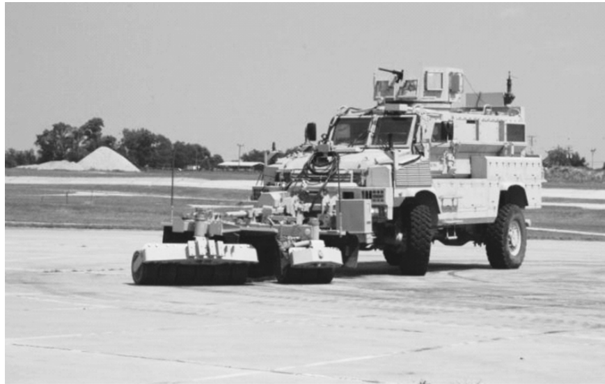
Figure 10. MRAP Vehicle with Forward Full-width Rollers (OEF) Installed (DoA, 2009, p. 002-3)
