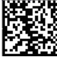
Figure 3. Data Matrix ECC200 (a.k.a., UID)
