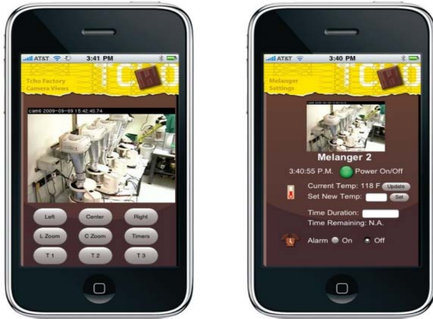
Figure 5. Smart-Phone (iPhone)–Based Views for Monitoring and Controlling Devices in a Physical Factory (Back, Kimber, et al., 2010)
