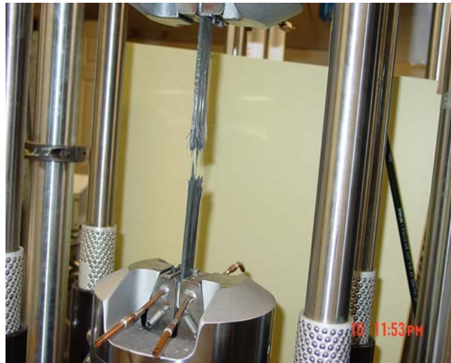
Figure 2: Specimen in The test fixture after fatigue failure.
