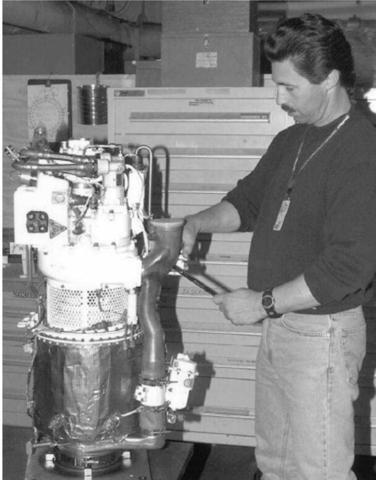
Figure 2. Employee performs repairs on an APU
