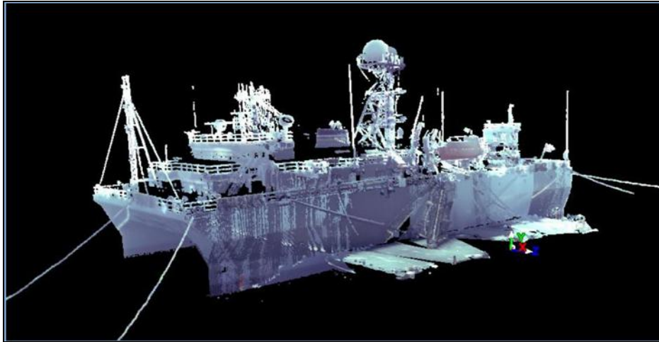
Figure 12. Sample Point Cloud Image (USNS Ship Exterior)
