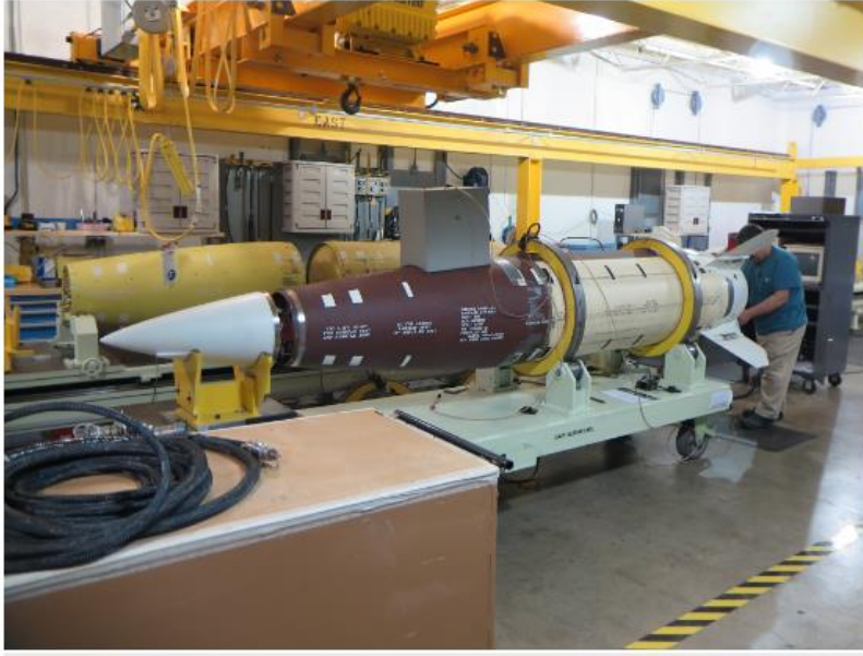
A Letterkenny Munitions Center employee disassembles an Army Tactical Missile. Letterkenny was named a Center for Industrial and Technical Excellence for Missile Maintenance in 2015 (Barati, 2015).
