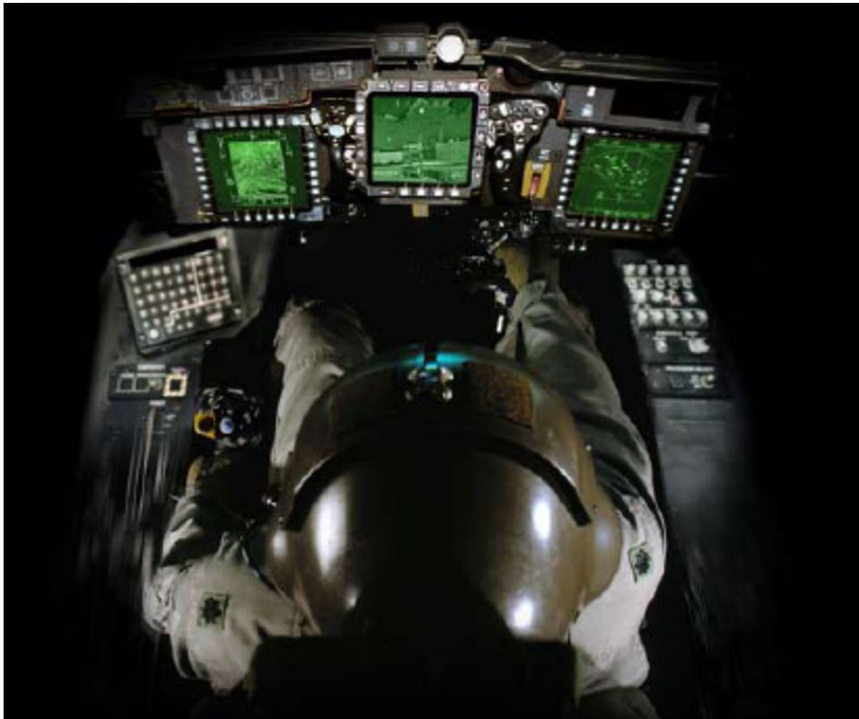
Figure 1. Multi-Purpose Displays in the Cockpit of an Apache Longbow Helicopter. Source: Lockheed Martin (2018).
