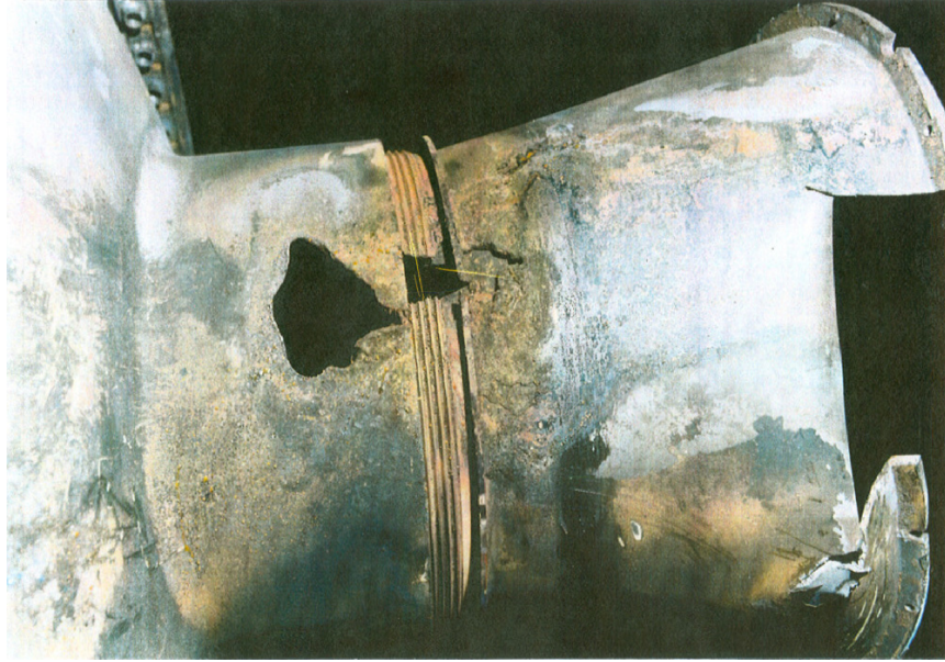
Figure 12. ATACMS Nozzle Exit Cone Assembly Burn-through
