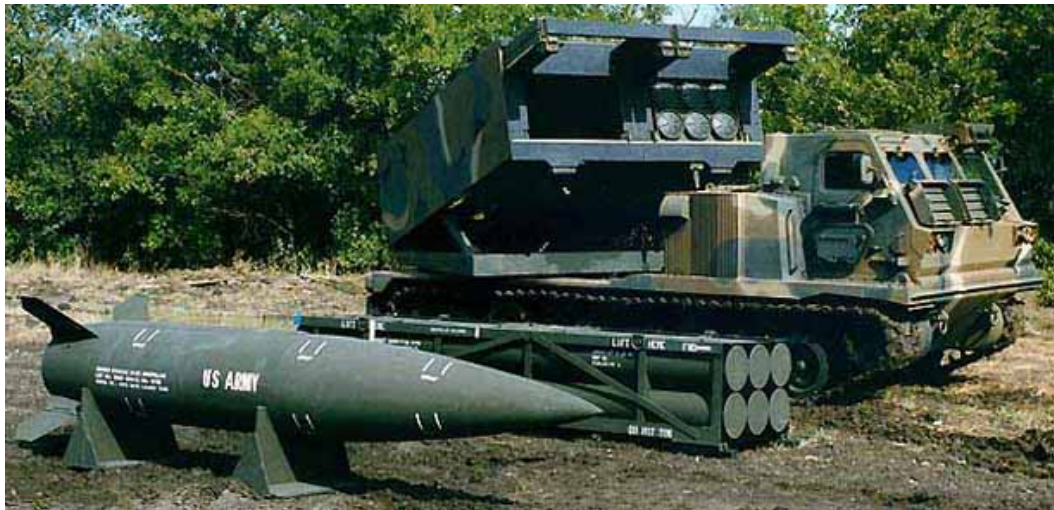
Figure 10. The Army Tactical Missile System Components Launcher, Missile, and Missile Launch Pod Container
