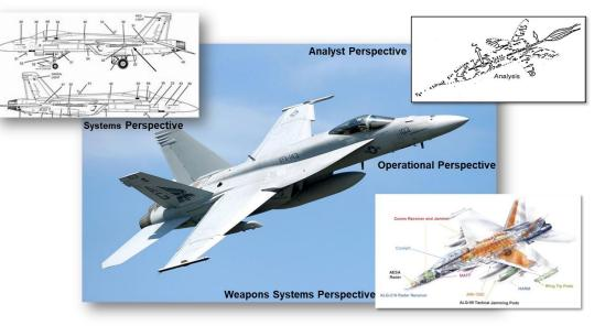
In a MBSE-environment CONCORDANCE the ability to represent a single entity such that data in one view, or level of abstraction, matches the data in another view, or level of abstraction, when talking about the exact same thing.
