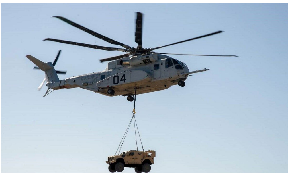
Figure 1. CH-53K King Stallion lifts a JLTV during testing demonstration in Patuxent River, MD. Source: Snow (2018).
