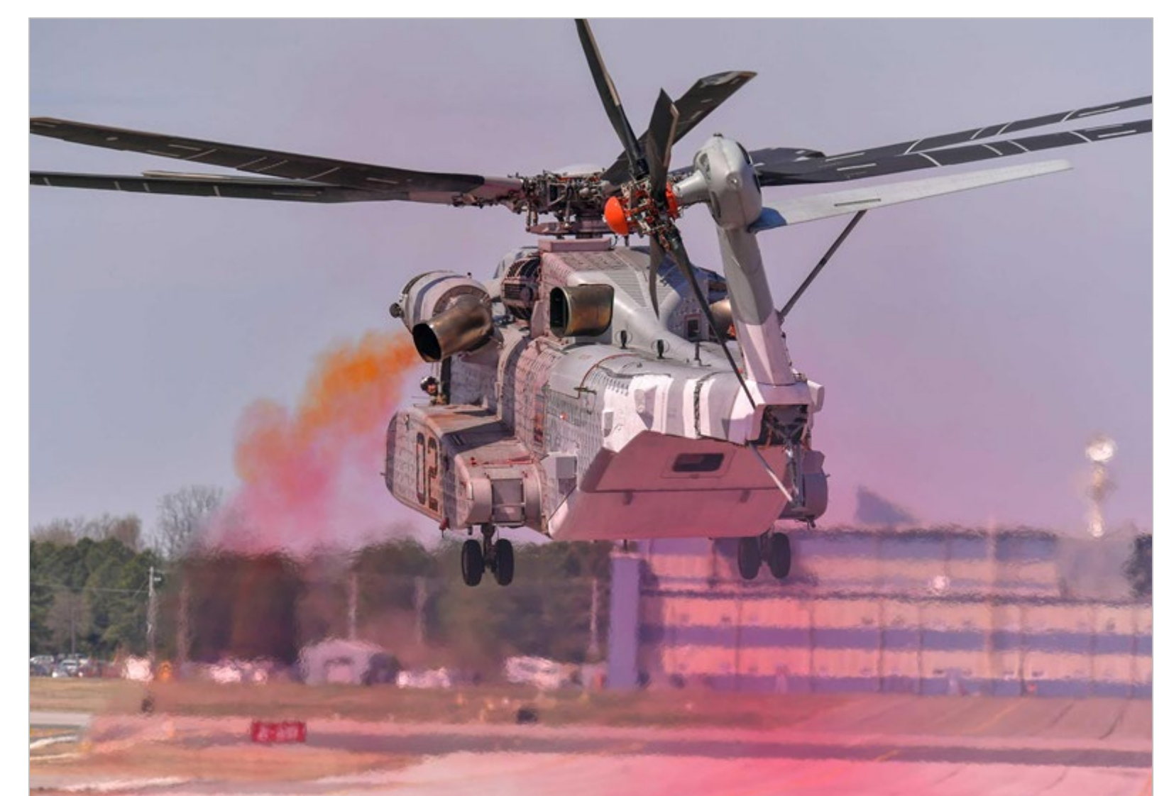
Colored oil smoke test identifies cause of engine gas re-ingestion issue on CH-53K.
