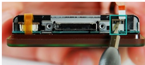
Image 16: Zune Battery Release
