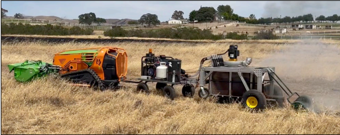
Figure 13. Demonstration of Burnbot Being Utilized to Create a Fire Break in a dense Dry Environment aboard Camp Roberts, CA (2022).
