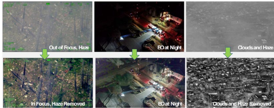
Figure 6. Vendor A Capability—GPU-Accelerated Multifilter Image Processing
