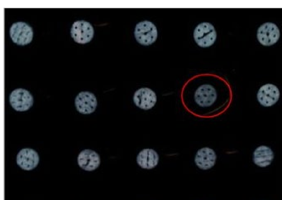
TM: HES 5808 Internal Cracking
