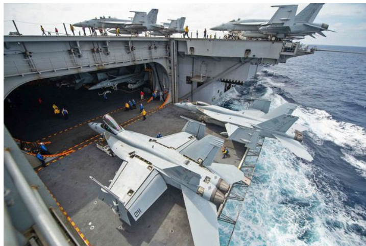
Figure 18. Hanger Bay Door and Elevator. Source: USNI (2006).
