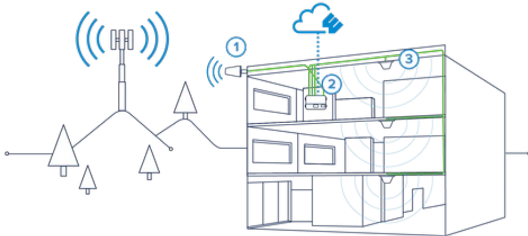
Figure 5. Spidercloud Cellular Signal Amplifying System Diagram. Source: Ekho Comm (n.d.).
