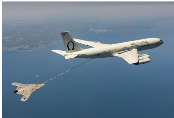
Figure 1. X-47 Conducts A3R Using Drogue Method. Source [8].
