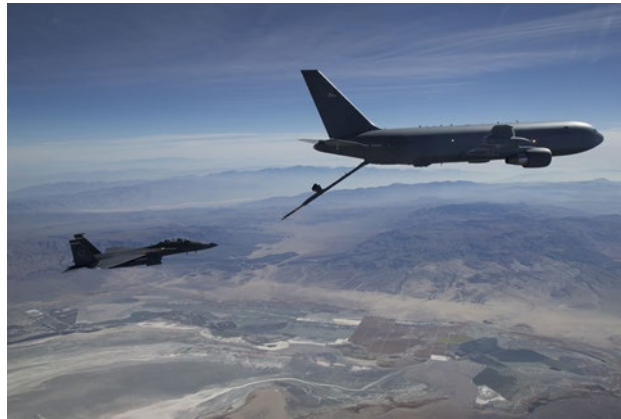
Figure 9. KC-46A Boom Refueling an F-15E. Source [18].
