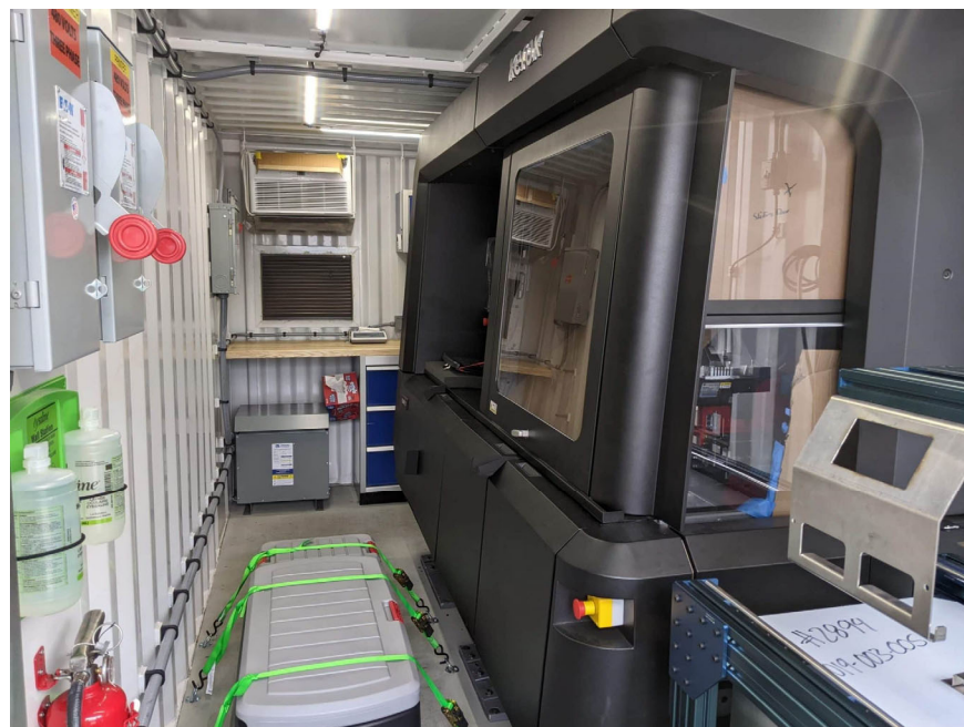
Figure 11. Interior View of Xerox ElemX Liquid Metal 3D Printer Installed in an 8' x 8' x 20' ISO Container for Use and Experimentation on USS ESSEX, July 2022. Source: Wakefield (2022).
