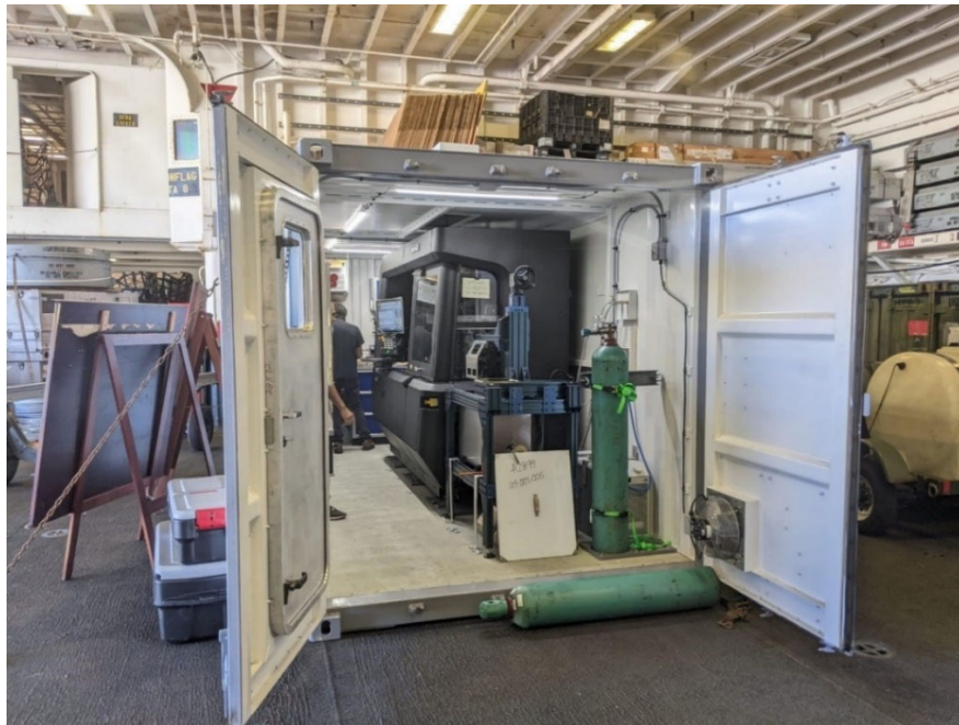
Figure 10. Xerox ElemX Liquid Metal 3D Printer Installed in an 8' x 8' x 20' ISO Container for Use And Experimentation on USS ESSEX, July 2022. Source: Wakefield (2022).
