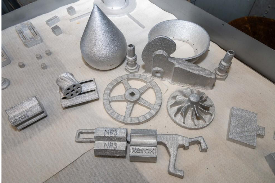
Figure 9. Aluminum Parts Printed at Naval Postgraduate School on the Xerox ElemX printer. Source: Martin (2023).
