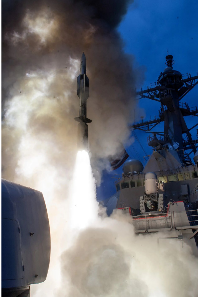
Figure 4. A Mk 72 Booster in Use during a Standard Missile 6 (SM-6) Launch. Source: Hempel (2016).
