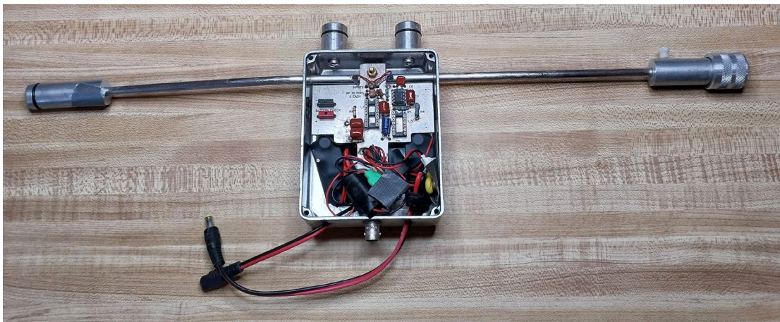
Figure 1. Original Walters Probe with a Fixed Separation of 50 cm Between Thermocouples
