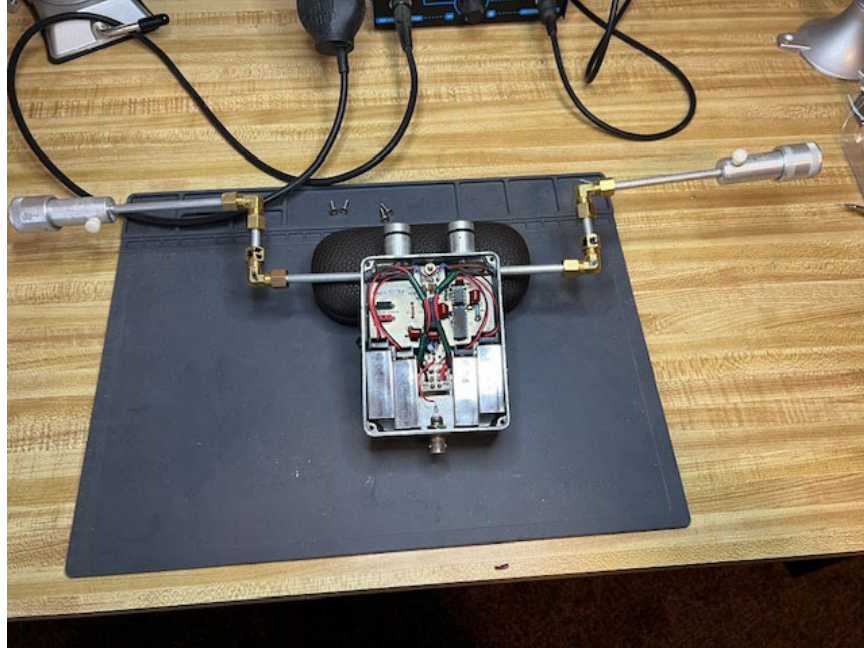
Figure 2. Interim Variable Separation Test Prototype with Thermocouple Arms Extended to maximum Separation
