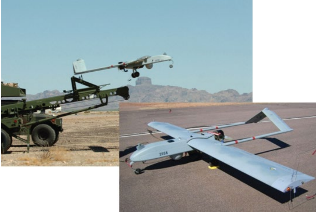
Figure 1. RQ-7 Shadow and launching mechanism Source: DOT&E (2010).
