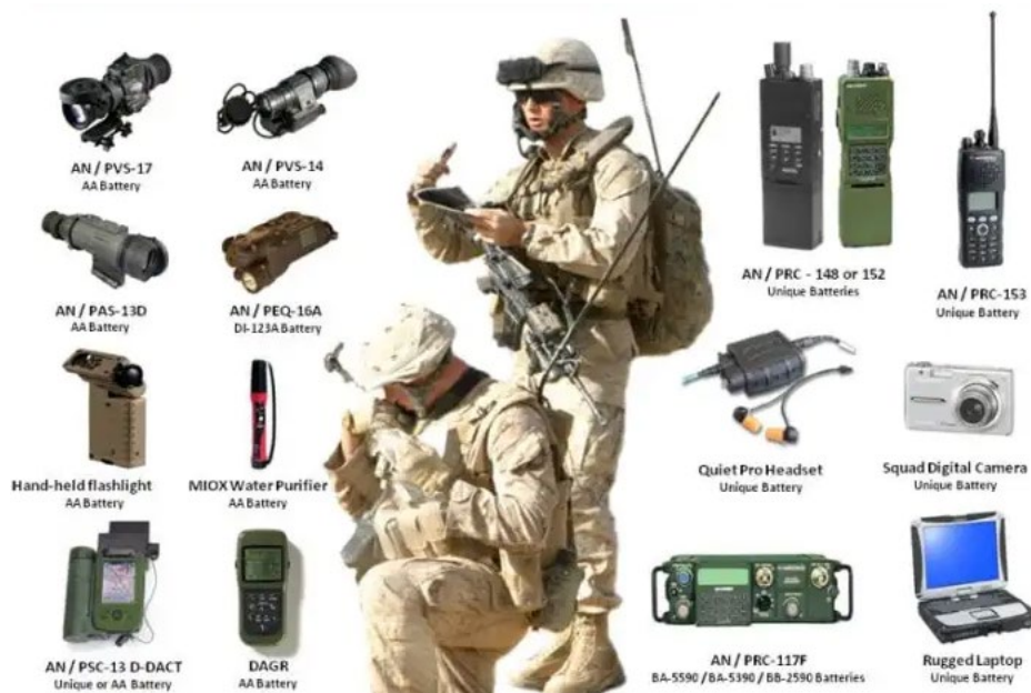
Figure 1. Individual marine power requirements. Source: Wilson (2010). This graphic shows the breadth and depth of energy required for a single soldier in the current age.
