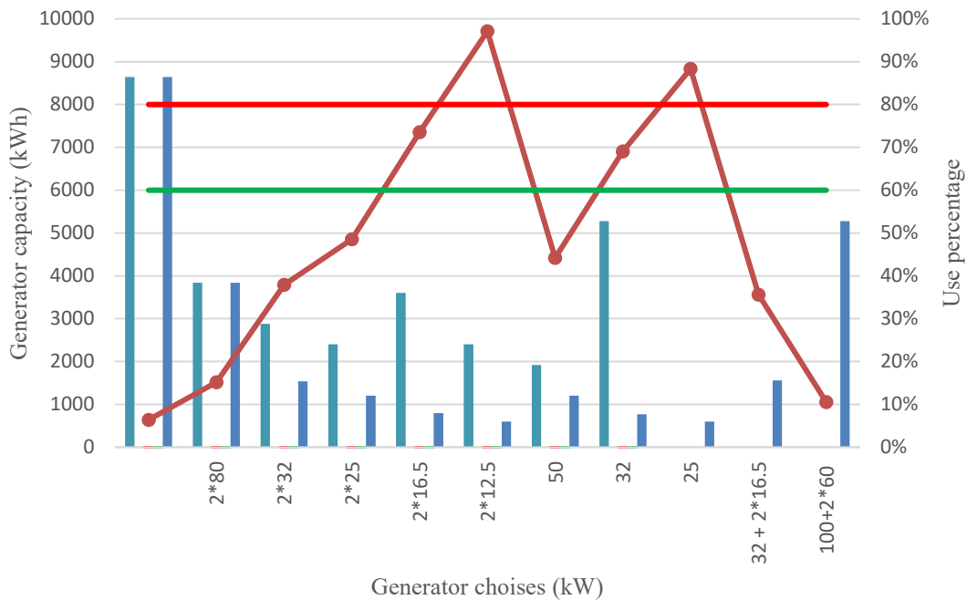
Figure 10. The generator choices in the “Sunny day in an urban area” scenario. The lower threshold (green) is 60 % and the upper (red) is 80 %.
