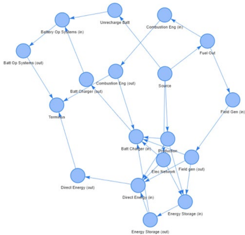
Figure 7. Unit's operational energy network. The nodes represent the source of energy, the conversion of energy, and the consumption of energy. The arcs represent the flow of energy. The Source and Terminus nodes are needed to create a feedback loop.
